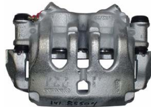
141.85504 Bore: 52mm Bleeder: 10x1mm Port: 10x1mm Pad: 10x.12680 Loc: Rear Pos: Trailing C# 929400
