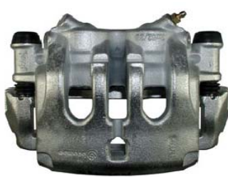
141.85002 Bore: 52mm Bleeder: 10x1mm Port: 10x1mm Pad: 10x.12680 Loc: Front Pos: Leading C# 929305
