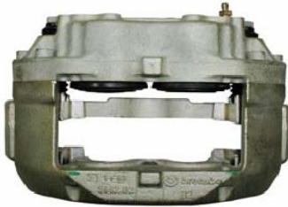
141.85501 Bore: 68mm Bleeder: 12x1mm Port: 12x1mm Pad: 10x.10270 Loc: Front Pos: Leading Brkt Cst: 5663.01 C# 566101
