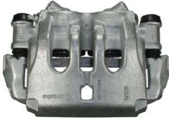
141.85001 Bore: 52mm Bleeder: 10x1mm Port: 10x1mm Pad: 10x.12680 Loc: Front Pos: Leading Brkt Cst: 929400 C# 929300
