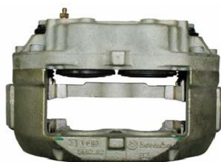
141.85502 Bore: 68mm Bleeder: 12x1mm Port: 12x1mm Pad: 10x.10270 Loc: Front Pos: Leading C# 5662.02
